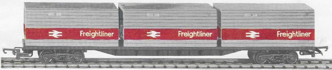
R.632 B.R. FREIGHTLINER WAGON with three 20-foot Open B.R. Freightliner Containers.
